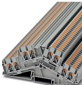
Double-level terminal block, nom. voltage: 800 V, nominal current: 20 A, connection method: Push-in connection, 1st and 2nd level, Rated cross section: 2.5 mm<sup>2</sup>, cross section: 0.14 mm<sup>2</sup> - 4 mm<sup>2</sup>, mounting type: NS 35/7,5, NS 35/15, color: gray
