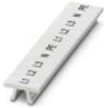
Zack marker strip, Strip, white, labeled, horizontal: L1, L2, L3, N, PE, L1, L2, L3, N, PE, mounting type: snap into tall marker groove, for terminal block width: 5.2 mm, lettering field size: 5.15 x 10.5 mm, Number of individual labels: 10
